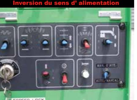
Stones that block the material feeding system can be ejected easily by reversing the feeder's direction using only a single switch.
