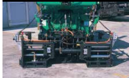
Height differences between main screed and extensor parts can easily be adjusted using the ratchet-lever of the new screed.
