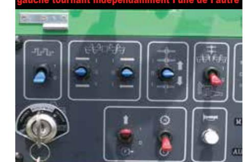
Being able to independently switch between forward and reverse movement of right and left auger ensures optimum volume of material.
