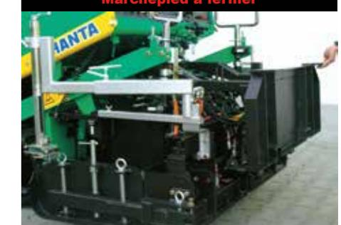
The operator's stand can be folded easily, when paving has to be started close to a wall.
